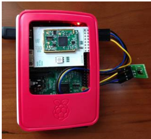
Figure 6: Raspberry Pi2 mini-computer with carbon dioxide and temperature sensor.
